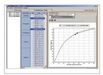
CT Saturation Curve Test Result
